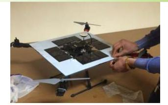
Figure 2 Position setting of the solar cells on the drone
