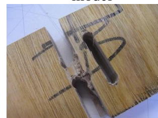
MACU plywood tension testing (CIB Weimar) 2014
