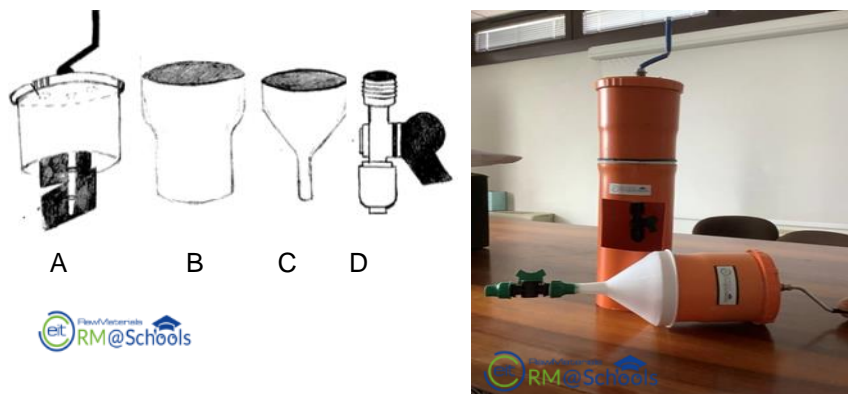
Figure 2. The picture on the left illustrates the individual components of the reactor: A) lid; B) central body; C) funnel; and D) Tap. The image on the right displays the mounted reactor
