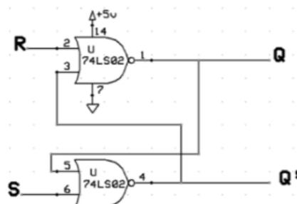
**Fig 3.** Physical Circuit Schematic of RS-Latch using NOR Logic Gates.
