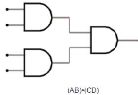
**Fig. 1** Schematic of a 4 input AND gate created in lab 1.
