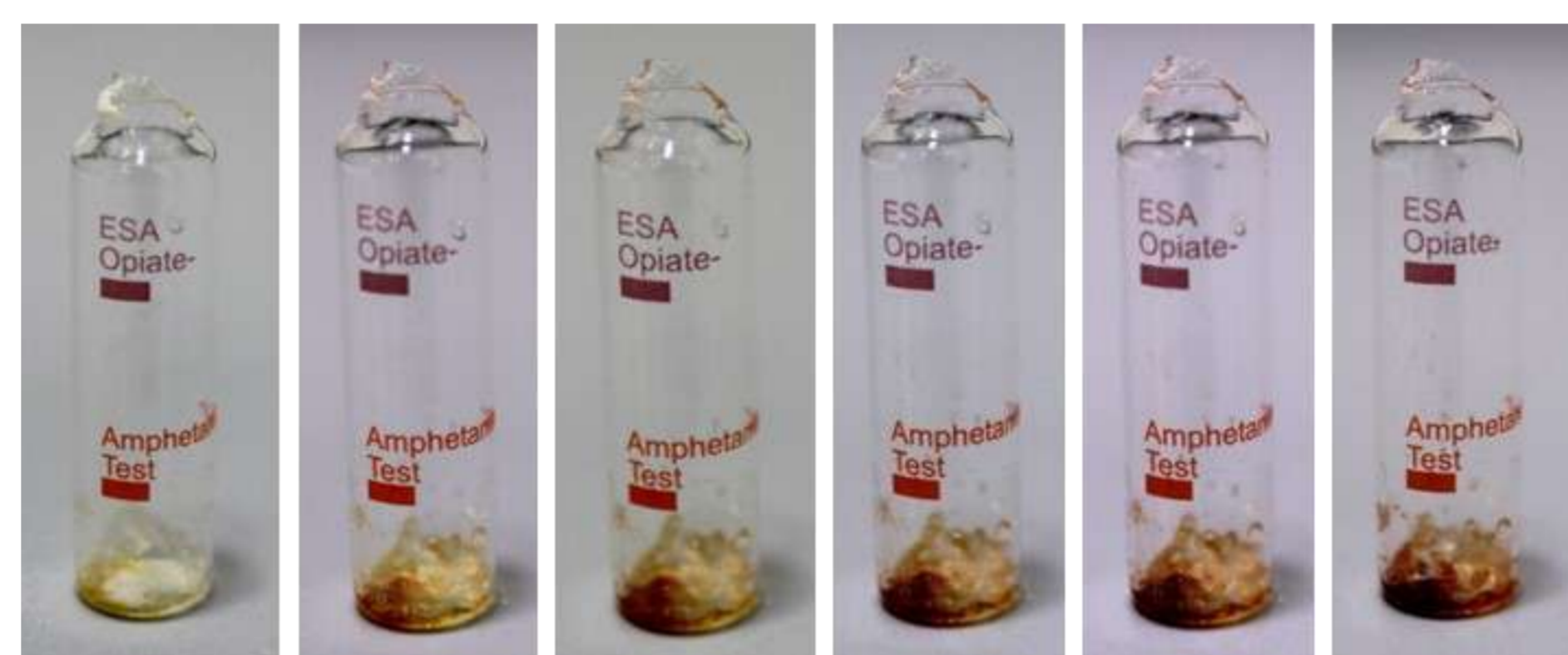
Figure 4: Course of the color reaction when adding amphetamine or methamphetamine to the Marquis reagent (from left to right: after 10, 30, 60, 120, 180 and 240 seconds); own photography (taken on 20.12.2017)
