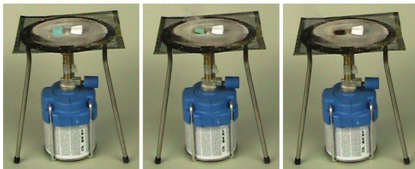
Fig. 6. Demonstration of the heat resistance of a mesoporous silicone (right) in comparison to an ordinary household sponge (left).
