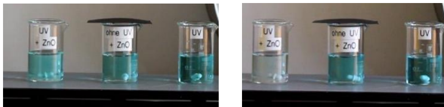
Figure 7: Photocatalysis of a green malachite solution with UV-light, UV-light and zinc oxide nanoparticles and without any of them in comparison
