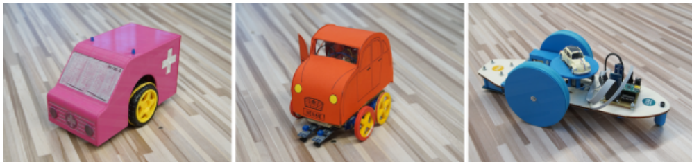
Fig. 4. Various line follower designs. Robots differed in wheel diameter, number of infrared sensors and the placement of the sensors
