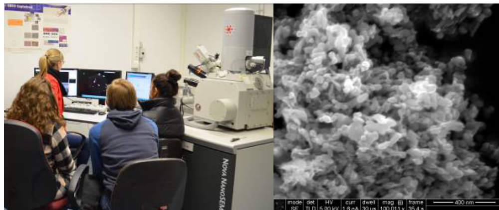
Fig. 2. Left: School students at the SEM. Right: SEM image of \text{TiO}_2 nanoparticles isolated from commercial sunscreen
