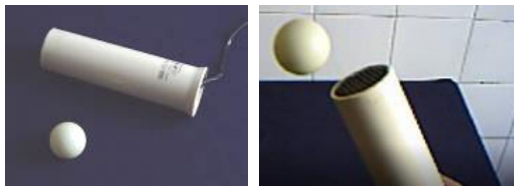
4. Figure: exploring Bernoulli's principle with hair dryer
