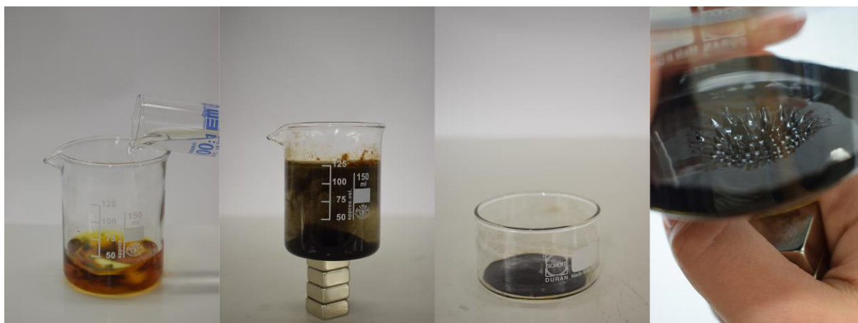
Fig. 2 from left to right: Solution upon addition of ammonia, sedimentation of nanoparticles with the magnet, washed nanoparticle dispersion, ferrofluid stabilized with TBAH.
