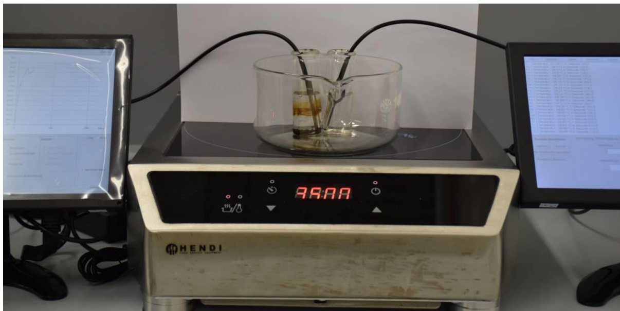
Fig. 3: Experimental setup: Induction hob with both vials. The left one contains a ferrofluid, the right one only water. Temperature measurements are acquired with LabPi measuring stations.
