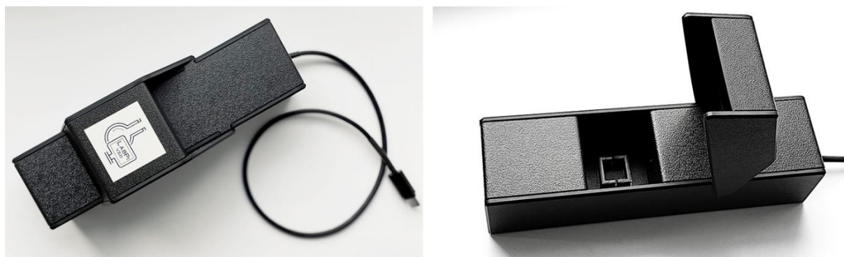
Fig. 1: Left: Image of the LabPi photometer with the measuring chamber closed. Right: Image of the LabPi photometer with the measuring chamber open and view of the holder for the cuvette.
