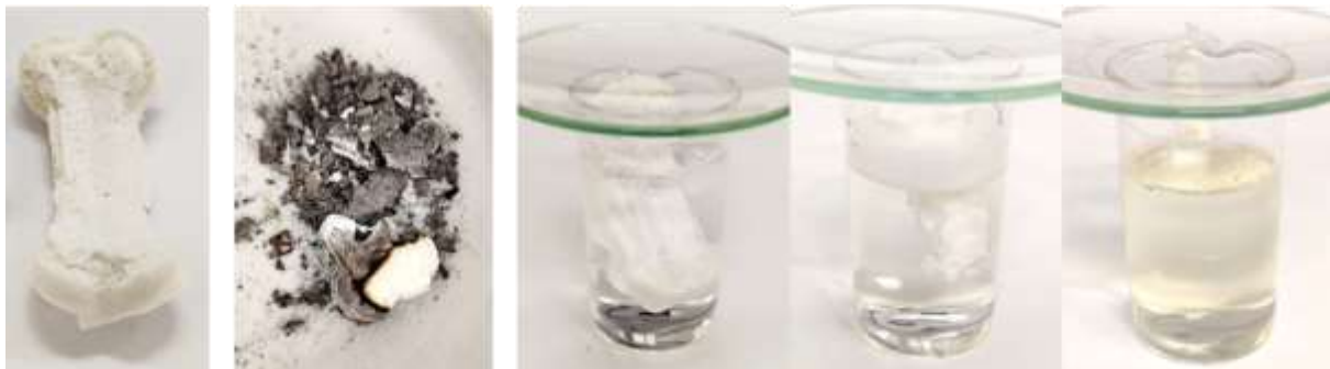
Fig. 6. Composite (left), after burning (center) and during incubation in 2 M HCl (right).
