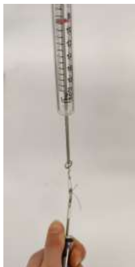
Fig. 1. Tensile strength measurement with a spring force meter.
