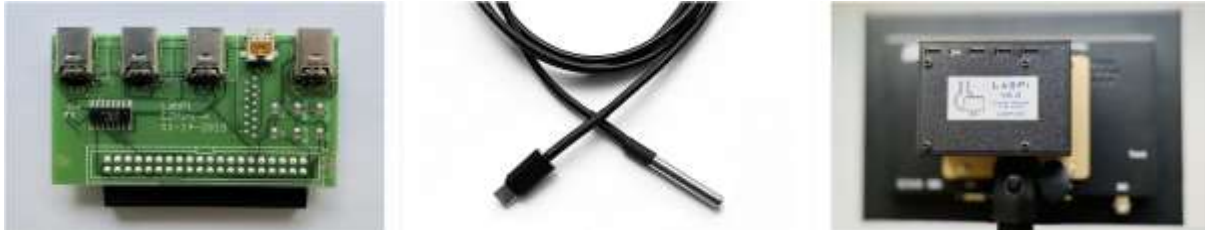
Fig. 1: Adapter Board (left), temperature sensor (middle) and the assembled LabPi-Station on a touch display (right).
