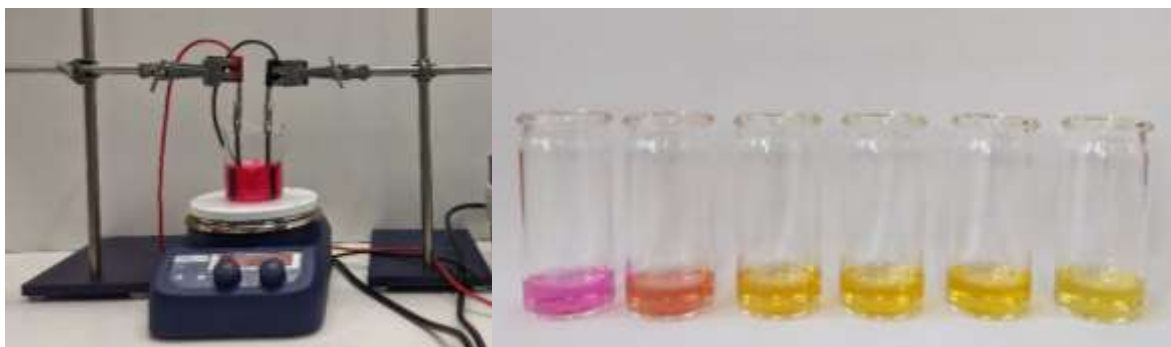
Fig. 1: Experimental Setup (left) and color change of the reaction mixture during electrochemical bromination shown on samples taken after 0, 3, 5, 7, 9 and 15 minutes, respectively (right).
