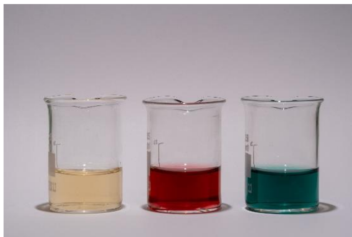
Fig. 2. Reaction mixture of KMnO_4 and KI in strongly acidic, neutral and strongly basic medium, respectively (left to right).
