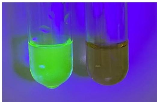
Fig.1. Left: fluorescein solution under UV illumination; Right: fluorescence of eosin Y as the product of electrochemical bromination of fluorescein.
