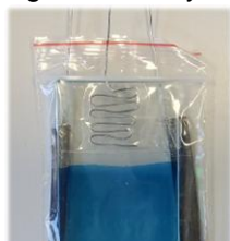
Fig. 3. Electrochromic window that can be used to regulate light and heat in buildings. It uses redox reactions ( \text{Fe}^{2+}/\text{Fe}^{3+} ) based on Prussian blue and the incorporation of ions to change its colour reversibly. Foto: Scharmann, Lehmann
