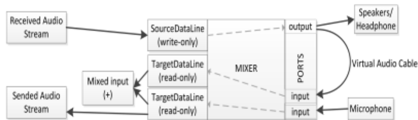
Fig. 4. Schematic of audio system implemented
