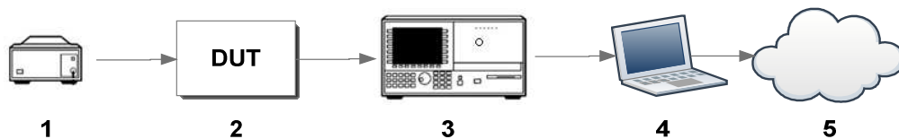
Fig 3. Real experiment layout: Light source (1), Device under Test, DUT (2), (3) Optical Spectrum Analyzer, OSA (3), Computer (4), and Internet (5).
