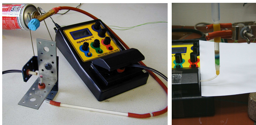
Fig. 2. The Spektra TM spectrometer upgraded into a simplified gas chromatograph (left) and a liquid chromatograph (right).
