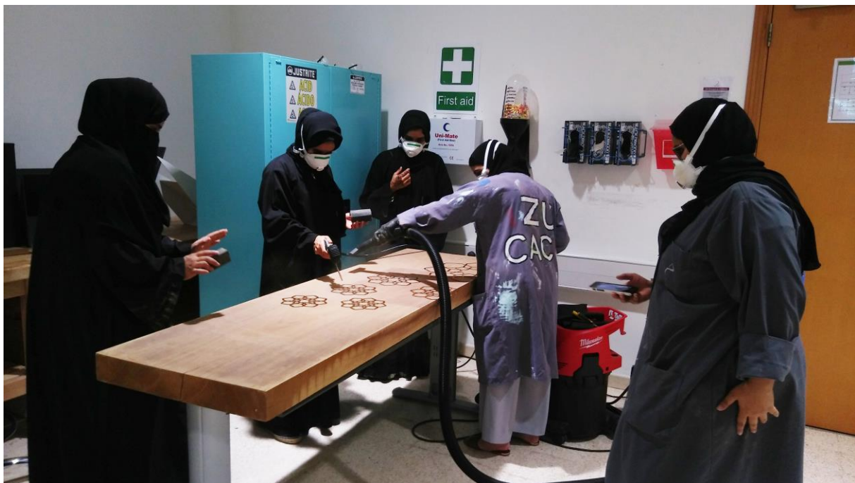
Fig.2. Students cleaning a robotic engraved pattern with compressed air, Prof. Thorsten Lomker
