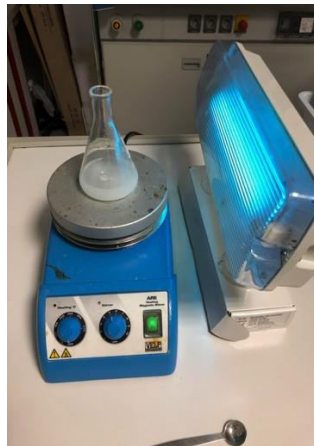
Figure 4. Experimental Set-up (bacteria solution in the presence of ZnO and UV light)
