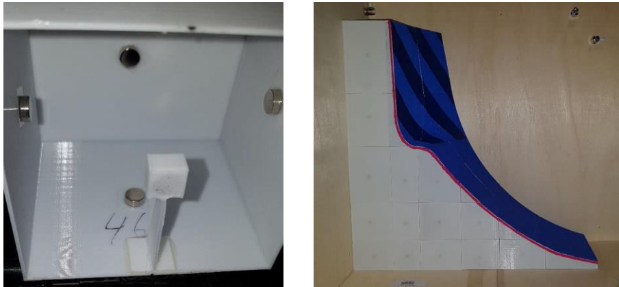
Fig.2: Inner side of a 3D printed hollow body of a single segment with round magnets for detachable cohesion (left); Critical isotherm on the opened model (pink line) (right) [1].
