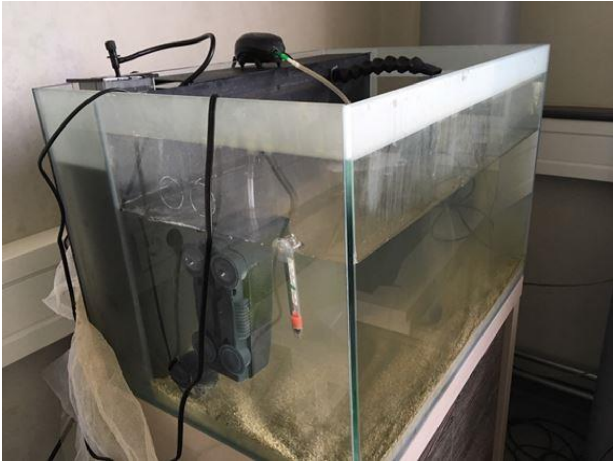
Figure 1: First set up of the aquarium as a test tank. You can see the skimmer in the technical chamber (far left), the mechanical internal filter (center), the thermometer (center), the pump for aeration (top center) and the circulation pump (top right), own representation.
