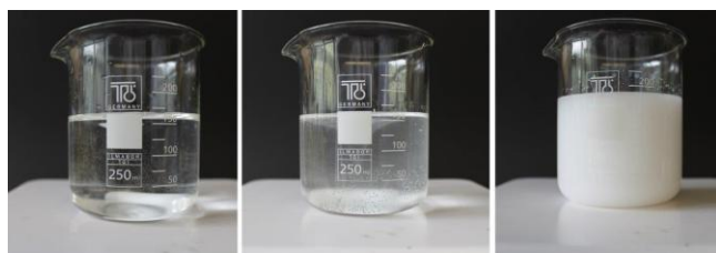
Fig. 2. Stages of the formation of formation of Stöber nanoparticles in a school experiment directly after addition of TEOS (left), after 20 minutes (centre) and after 24 hours (right).
