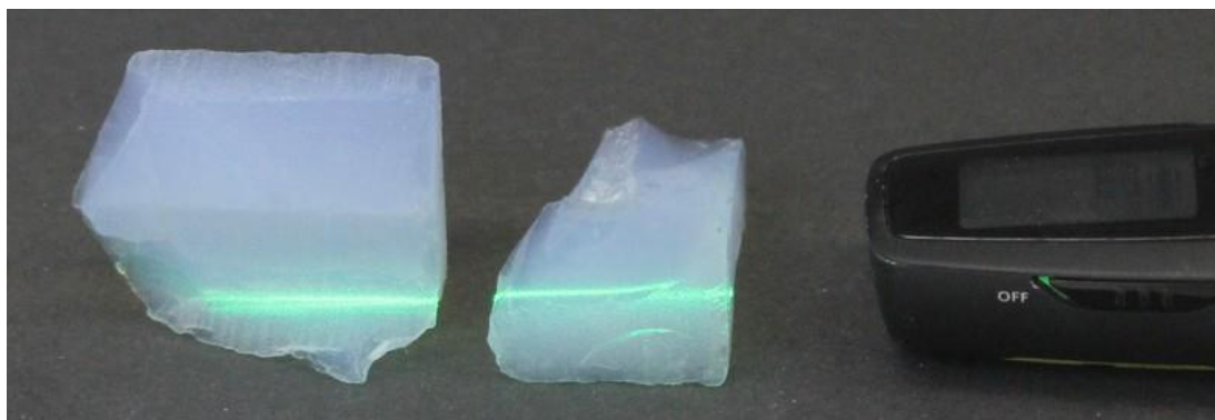
Figure 4: Visualization of a laser beam inside an aerogel.
