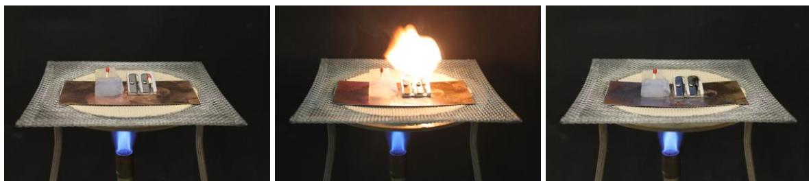
Figure 5: Demonstration of the thermal conductivity of aerogels and metals; matches after one minute (left), after three minutes (center) and after thirteen minutes (right).
