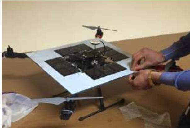
Figure 2 Position setting of the solar cells on the drone
