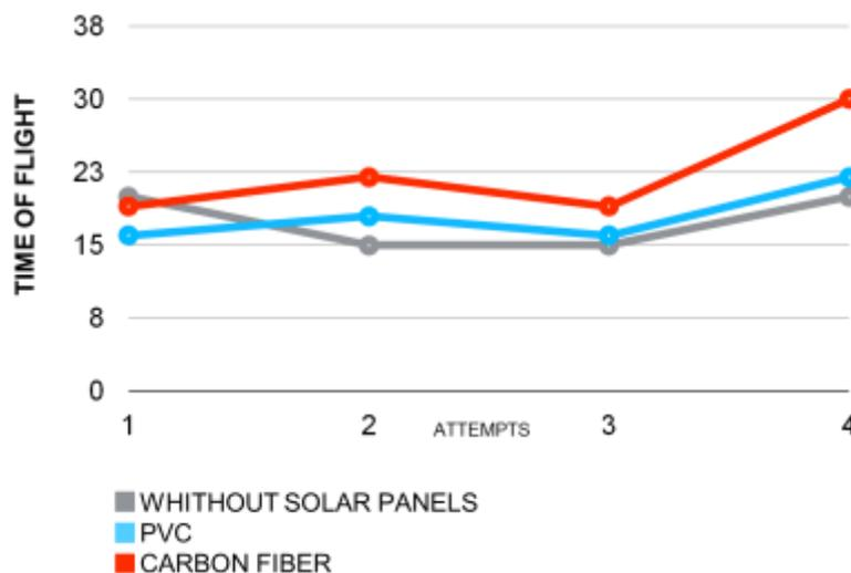
Figure 1: Time of flight of the drone in four attempts and with respect to building materials of the photovoltaic panels
