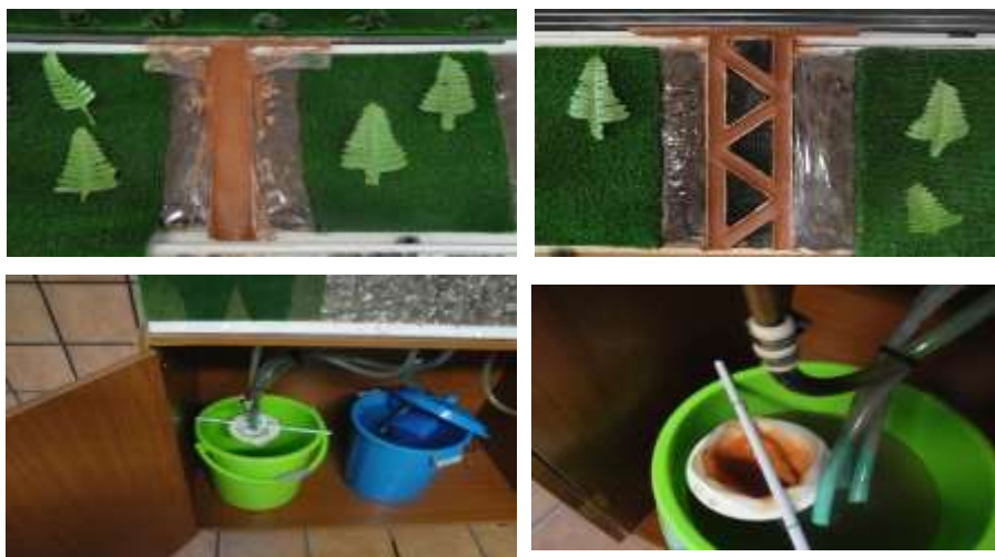
Fig. 3. Molded channels made in clay, water with sediments tank and collection filters.
