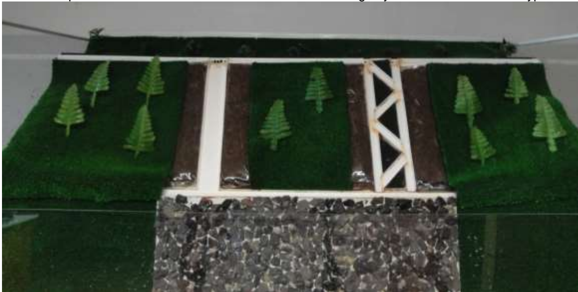
Fig. 1. Front of the model with two drainage system simulating the slope of a road.
