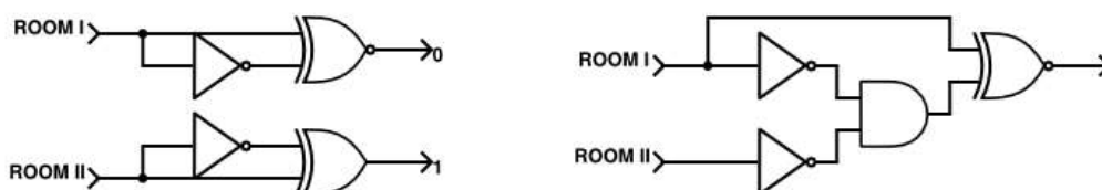
Figure 6. Testing of the upper sign (left) and reduced circuit of Trial 8 (right)
