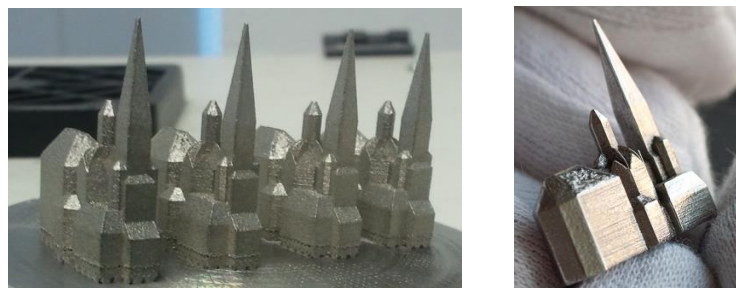
Fig. 4: Different materials left: printed model, metal printer (mild steel); right: model after manual polishing (silver)
