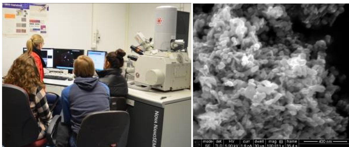
Fig. 2. Left: School students at the SEM. Right: SEM image of TiO 2 nanoparticles isolated from commercial sunscreen.
