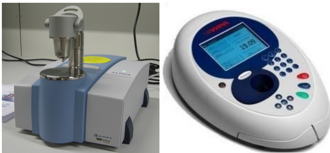
Fig 1. Left the IR spectrometer with ATR attachment and right the UV-vis spectrometer, both of which are used for SIAS workshops in the Republic of Ireland.
