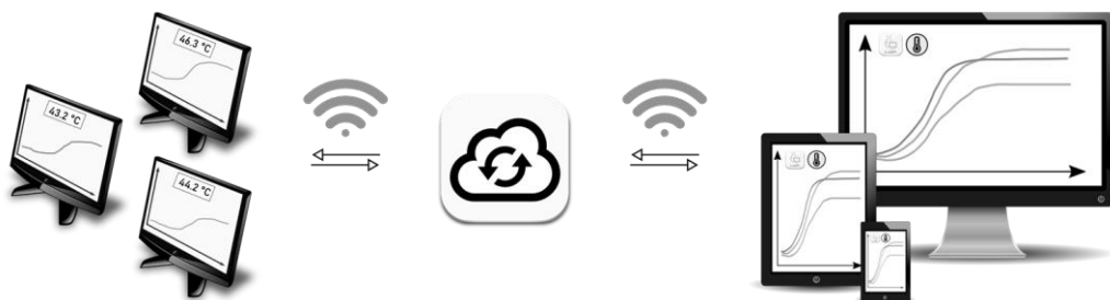
Fig. 4. Consolidation of the results from several LabPi stations (left) via the associated cloud platform COMPare as well as graphical representation on various display devices (right)
