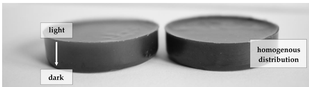
Fig. 3. Comparison of nanocomposites. Left: Without functionalization; right: with functionalization
