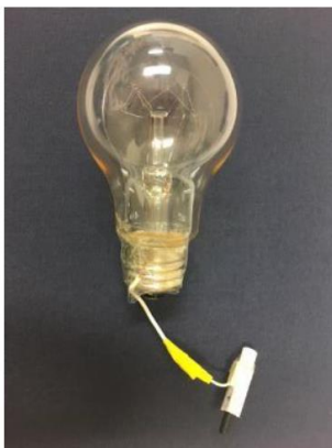
Fig. 3. Lightning test device using vibration-resistant bulb and piezoelectric device
