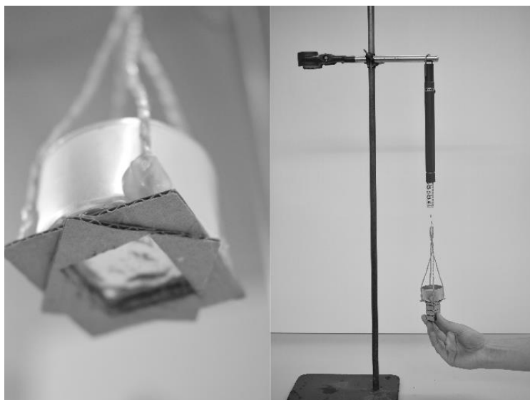
Fig. 4. Low Cost analysis for school chemistry education: Bowl to hang up the sample with attachment for the magnet (left); deflected force meter, during measurement (right)
