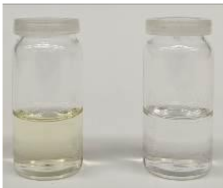
Fig. 2. left: solution after electrolysis; right: colorless solution after the addition of the alkene
