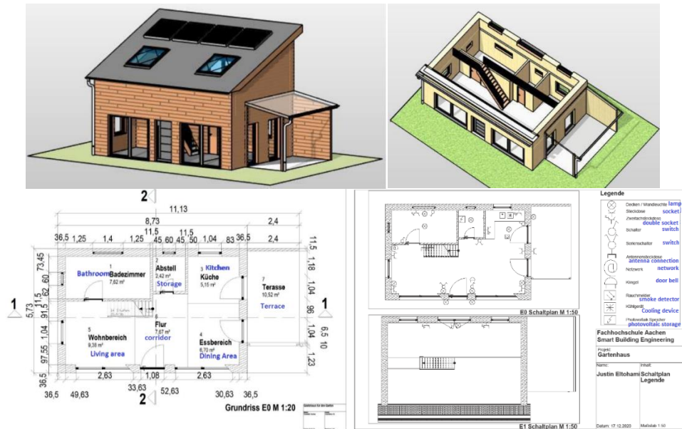
Fig. 1. Front view of the 3D model (top left), open top view of the 3D model (top right), floor plan (bottom left) and installation plan of one of the groups [4]
