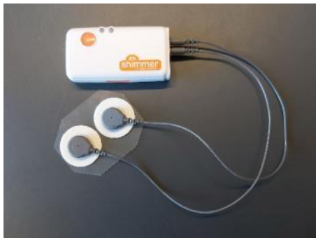
Fig. 2. Adapted sensor and Shimmer device for EDA measurement
