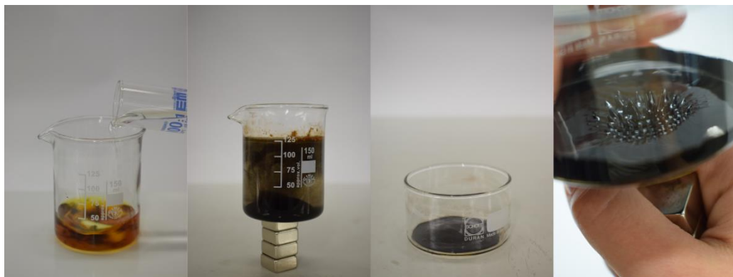
Fig. 2. from left to right: Solution upon addition of ammonia, sedimentation of nanoparticles with the magnet, washed nanoparticle dispersion, ferrofluid stabilized with TBAH.
