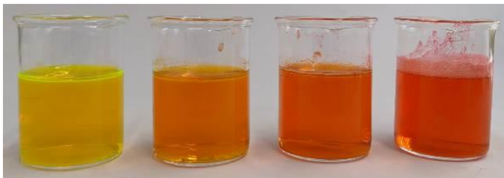
Fig. 1. Fluorescein solution, electrolyzed solutions after 30 seconds, 1 minute and 2 minutes, respectively
