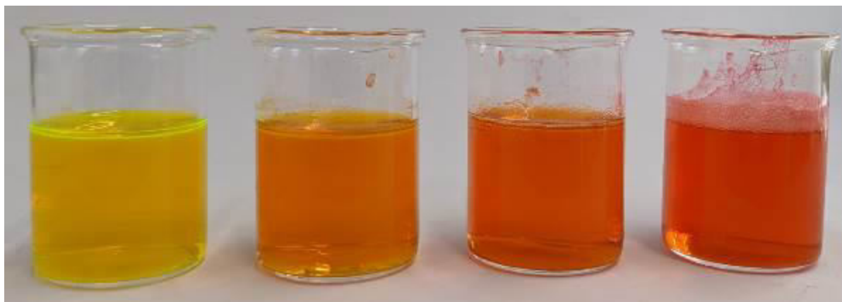
Fig. 1: Fluorescein solution, electrolyzed solutions after 30 seconds, 1 minute and 2 minutes, respectively.
