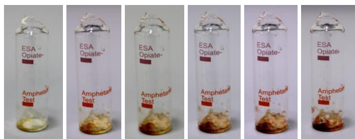
Fig. 3. Course of the color reaction (from left to right: after 10, 30, 60, 120, 180 and 240 seconds); own photography (taken on 20.12.2017)
