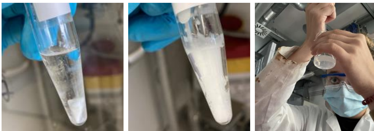
Fig. 1: Piloting of the experiments during Jena Summer School (2021). Start of reaction (ROP, left), Reaction mixture after 5 minutes (ROP, middle), student conducting the nanoprecipitation (right).
