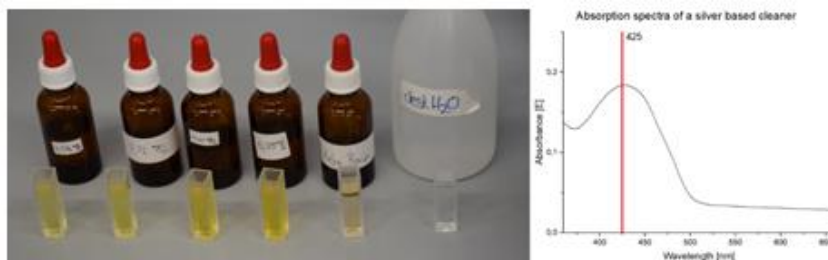
Fig. 4: Left: Dilution series and sample of the cleaner. Right: Recorded spectrum of the cleaner.
