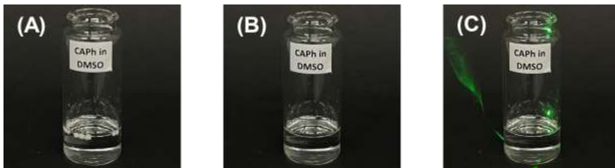
Fig. 2. (A): CAPH in DMSO before dissolving, (B): CAPH in DMSO after dissolving by stirring, (C): Negative Tyndall effect of CAPH in DMSO.
