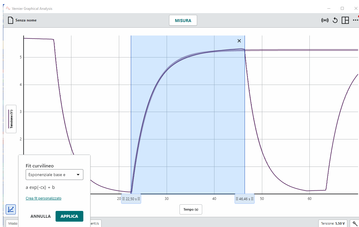
Figure 3: In order to perform a best fit with Graphical Analysis, first of all select the set of data involved; this can be done by highlighting the area directly on the graph.
