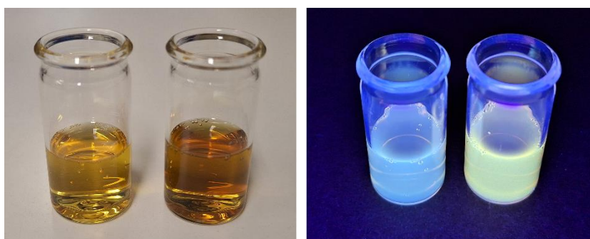
Fig. 2: Photography of the synthesized CQDs with a ratio of 3:1 (left) and 1:1 (right) citric acid and urea. The photo on the left was taken in ambient light and on the right under UV light ( \lambda = 365 nm).
